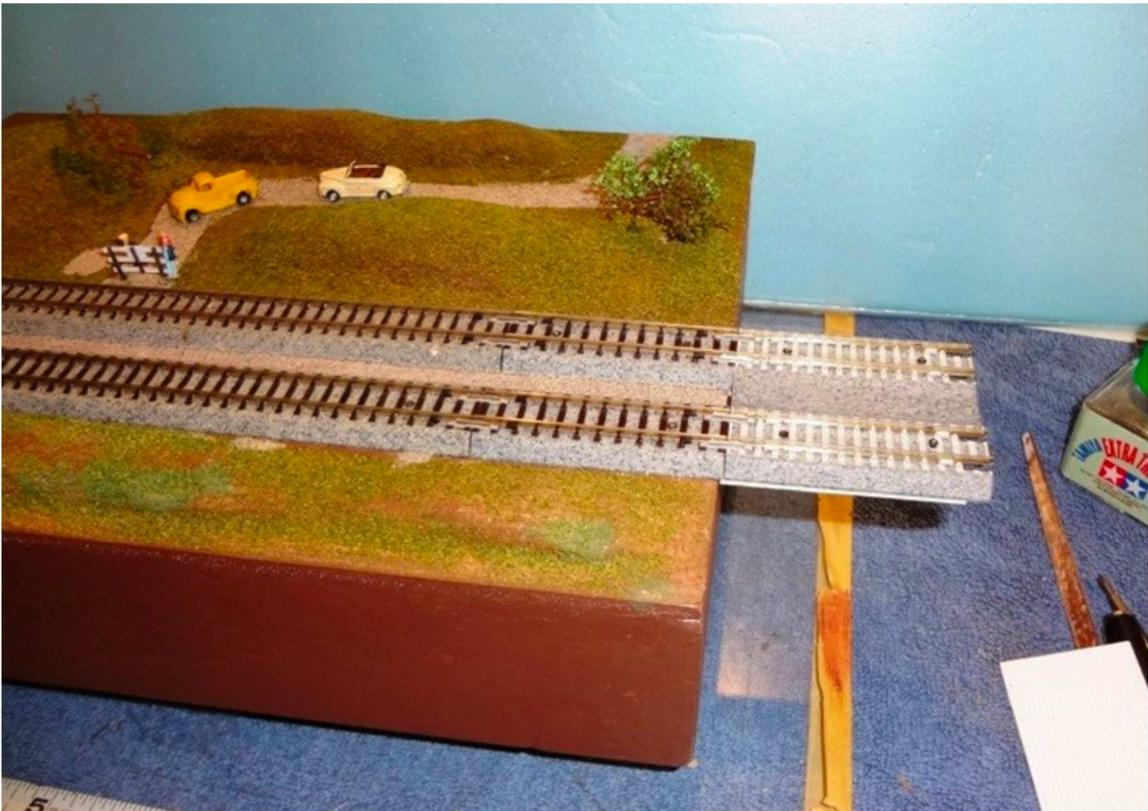
Finally, in Photo 4 you can see how the tool adjusts the edge of the track 1mm beyond the edge of the module. This allows the separation between modules to be 2mm, the standard separation.
